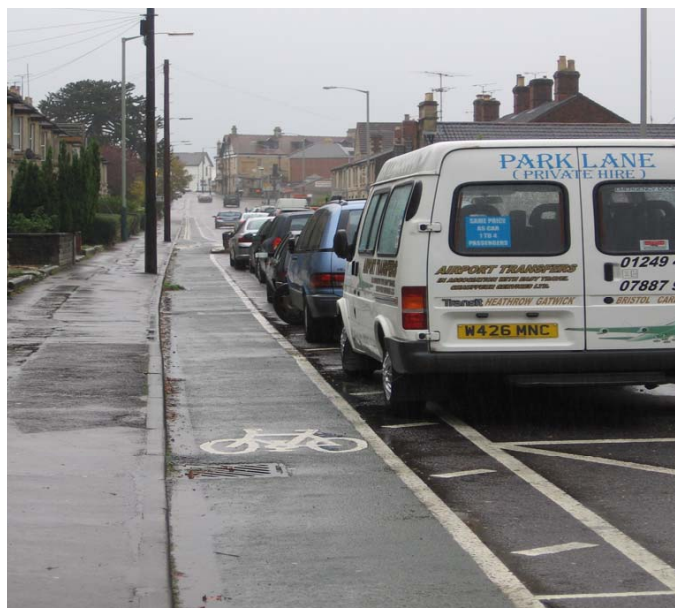
Picture 16.4 Mandatory cycle lane, New Road, Chippenham.
